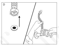
D. Make sure the filter screens are seated correctly in the hose fittings before connecting the hoses to the shutoff valves. Use an adjustable wrench to tighten the water supply hoses.
