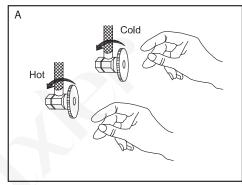
A. Shut off water supply at the valves. Remove old faucet and clean the mounting surface for installation of the new faucet.
