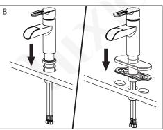
B. Use the Base Ring for a single hole installation OR use the included Escutcheon Plate to covert a 4 inch centerset hole pattern to a single hole installation.
