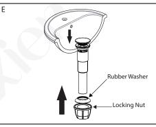
E. Remove rubber washer and locking nut from the drain assembly and slide the drain into the sink. Install the rubber washer first and tighten the locking nut to install the drain.
