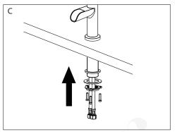
C. Under the sink, slide the washer and metal washer onto the faucet. Secure the faucet with the locking nut and screws to the countertop.
